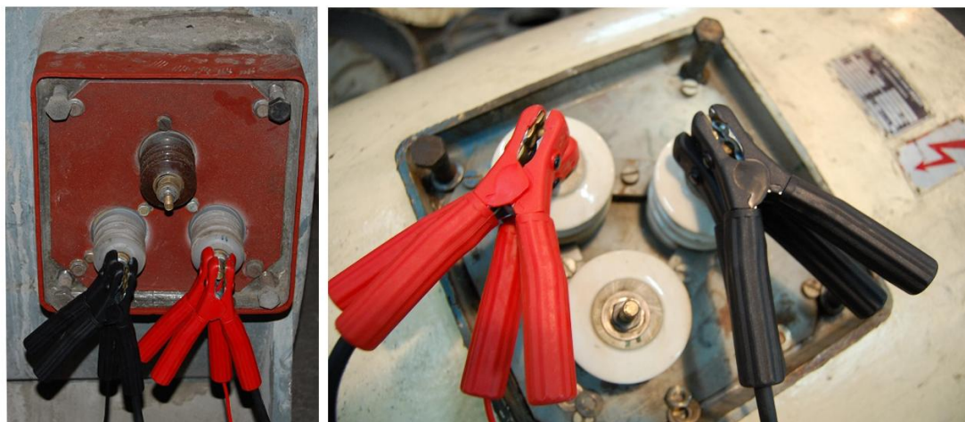
Figure 3: Connection for measuring the stator winding resistance of asynchronous motor
