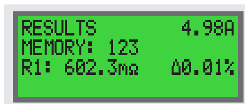
Figure 5: Example of the Results menu of RMO-M showing the test results
